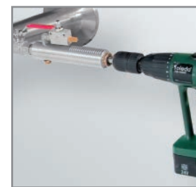
Drill under pressure with the CS Drill
